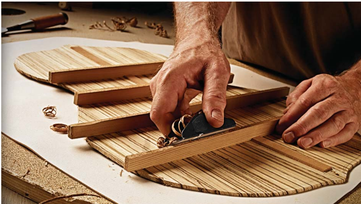
Stevens Point Luthier John Currier uses a hand planer to shape a brace for a guitar body.
