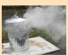
The fire is tended for several hours until extinguished and it's safe to remove the lid to ensure all the fuel has burned and the ceramics can be removed.
